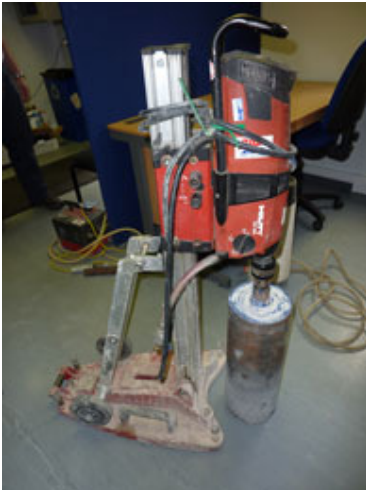
The core drill that the worker was asked to operate by hand
