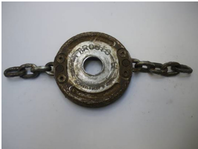
Chain flail attachment with two chains
