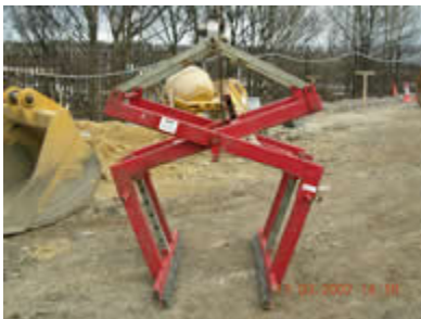
Block grab mechanism that was attached to an excavator and used to move a pallet of cement bags
